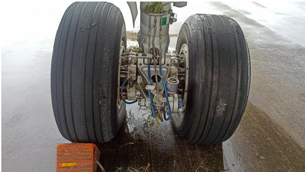
Fig 5: Cut marks on main wheel# 3 and 4 (front looking backward)
