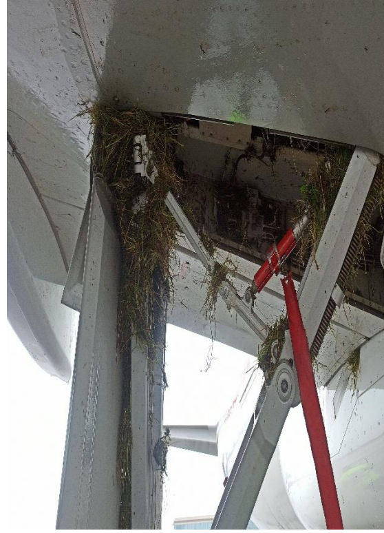
Fig 4: Grass ingestion at RH MLG
