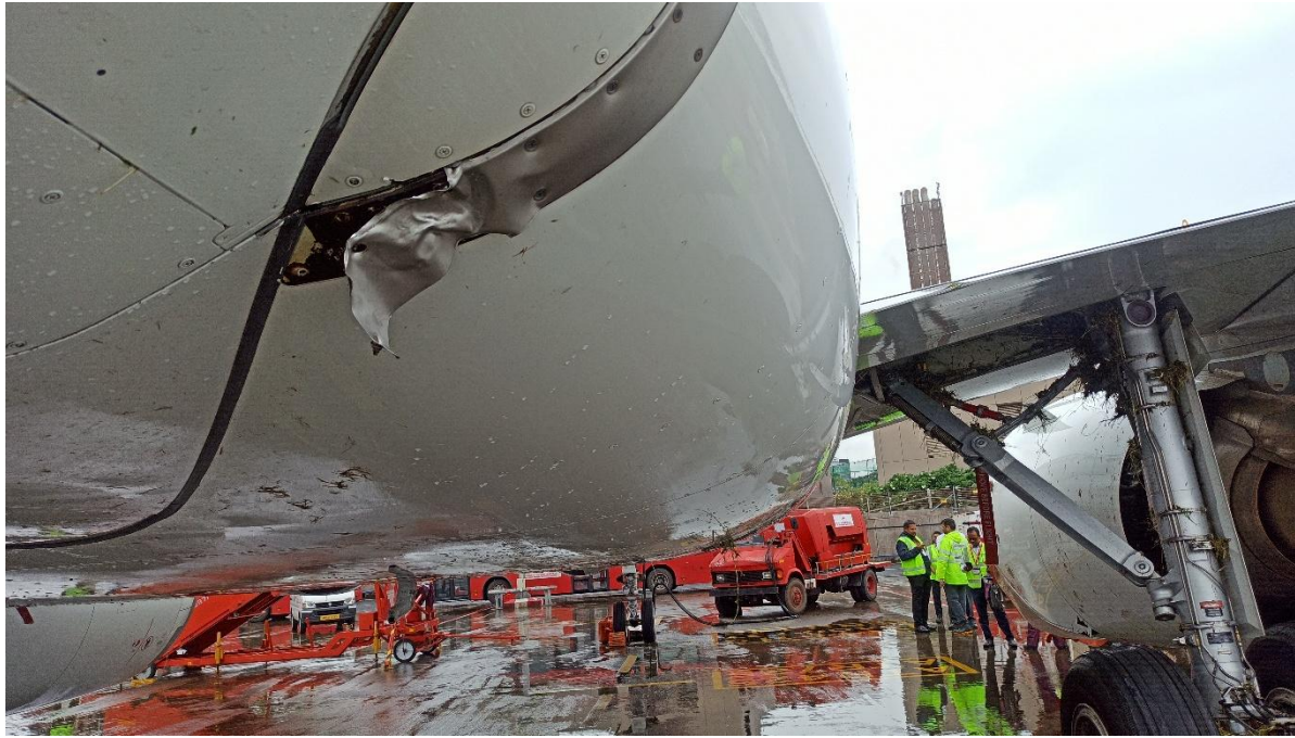
Fig 6: Damage to aft cargo 198BB panel fairing
