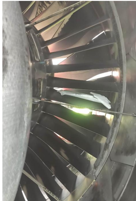
Fig 2: FOD ingested into bypass section of Engine# 2
