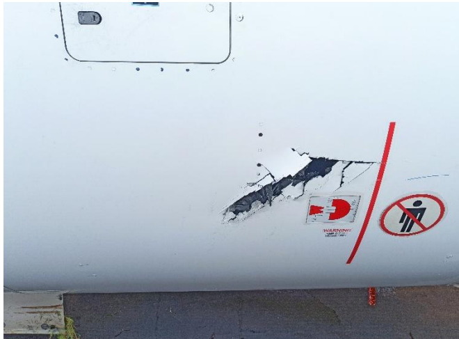
Fig 1: Damage to Engine# 2 cowling outboard side
