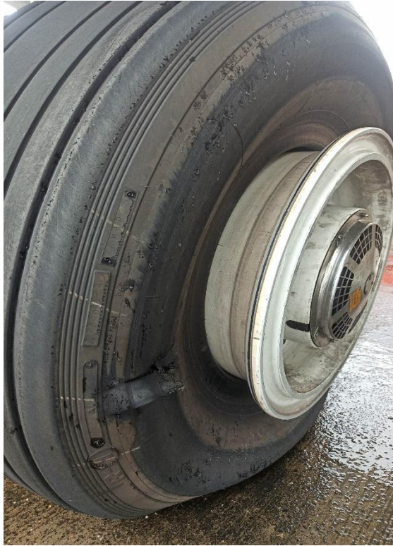
Fig 3: Cut mark on main wheel# 2
